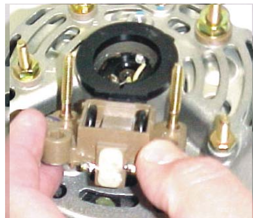
Installing Brush Assembly with Cover Screws and Rubber Seal
